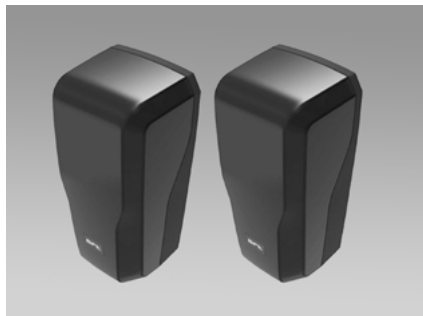
PHOTOCELLS – installed on the gate posts – whenever an object appears in the opening passage, the infrared beam is interrupted and movement stops.
