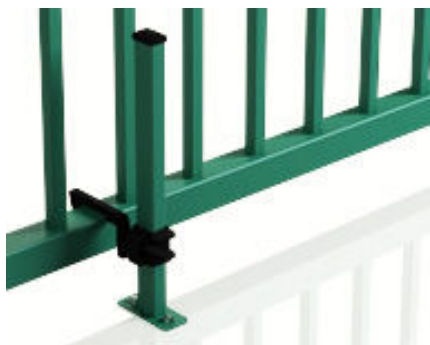
GRIPPING UNIT – prevents accidental closing of the opened leaf of the manually-operated gate, e.g. caused by a strong gust of wind. It is installed behind the gate and holds the leaves in the open position.
